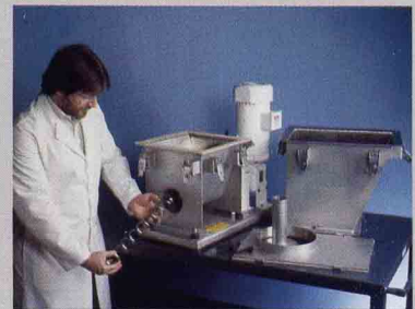
Figure 5. Feeder completely disassembled without tools and ready for cleaning.
