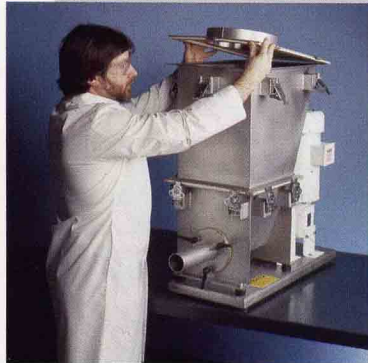
Figure 1. Hopper cover removed via quick-clamps.
