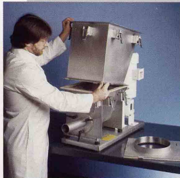
Figure 2. Hopper removed via quick-clamps.
