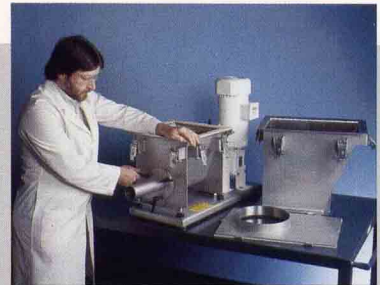
Figure 3. Feed tube removed by loosening ratchet hand clamps.
