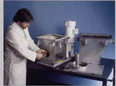
Figure 4. Feed screw unscrews and slides out.
