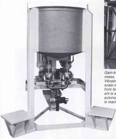
One of three loss-in-weight liquid batching bins for the manufacture of rocket propellants. High viscosity liquid is dispensed in 500 lb increments to a batch mixer. Thirteen other bins deliver up to two tons of dry ingredients each. Average accuracy of all Vibra Screw equipment is 0.05% of desired batch size.
